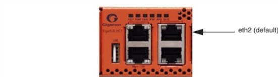
Figure 107 Stack Port Location on GigaVUE-HC1 Front
