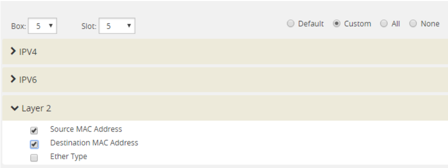
Figure 25 Advanced Hash with Source and Destination MAC Address
